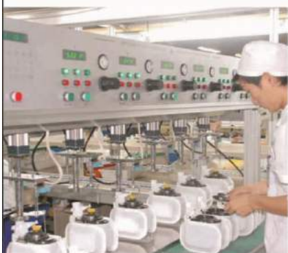
Automatic leakage test on measuring group
